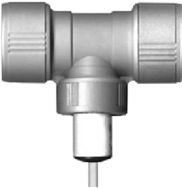
The tee sensor has been designed to go into the over flow pipes on break tanks, toilet cistern and header tanks. The sensor is located inside the tee piece and gets installed on the overflow pipe with the sensor at the bottom. Any water that travels down the pipe and into the tee sensor will make contact with the conductors of the sensor and set off the alarm.
